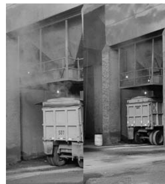
Figure 2 - Hopper Transfer Point - Fugitive Dust Comparison
