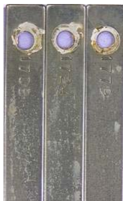
Figure 2: Comparison of Halogen Stable vs. Conventional Treatment, neutral pH, phosphate program, continuous chlorination (0.5 - 1.0 ppm free Cl 2 )
