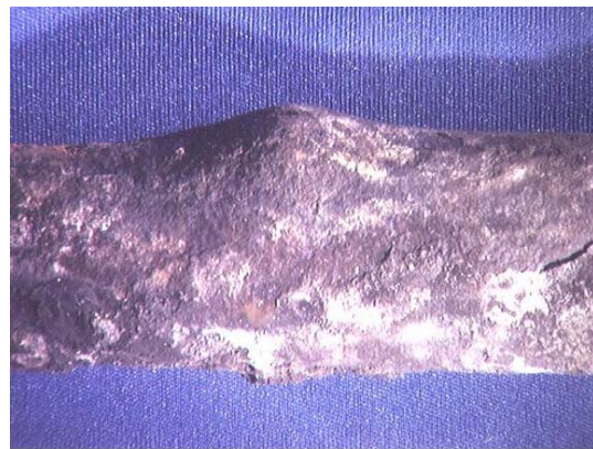
Figure 1 – Boiler water carryover formed deposits in this superheater tube and caused tube failure from overheating.
