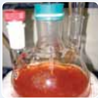
Glassware evaporator simulations on frac water before and after pretreatment
